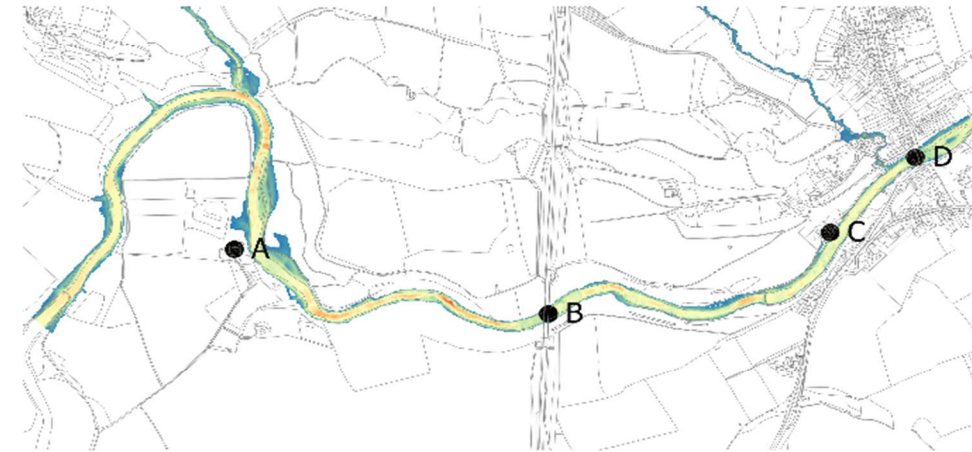
D) 10% AEP Scheme in Operation - Depth
