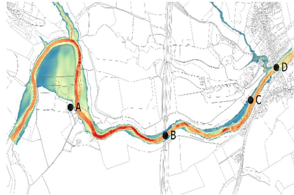
B) 0.1% AEP Scheme Construction - Depth
